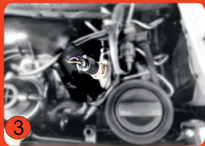
locate Common Rail sensor
